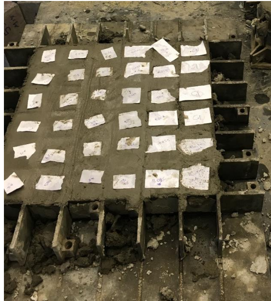
Figure 3-21: Mortar Cubes casted in molds
