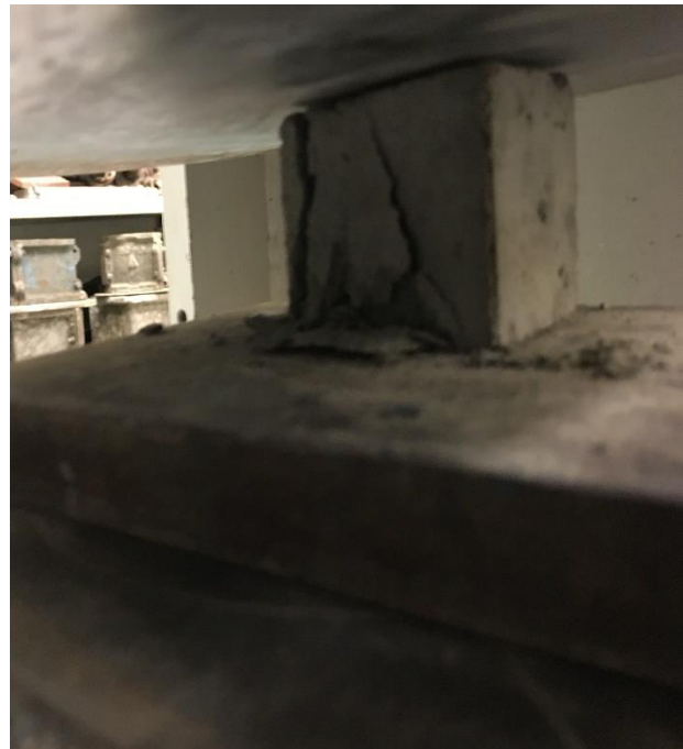
Figure 3-25: Cube fracture after applying ultimate compressive load
