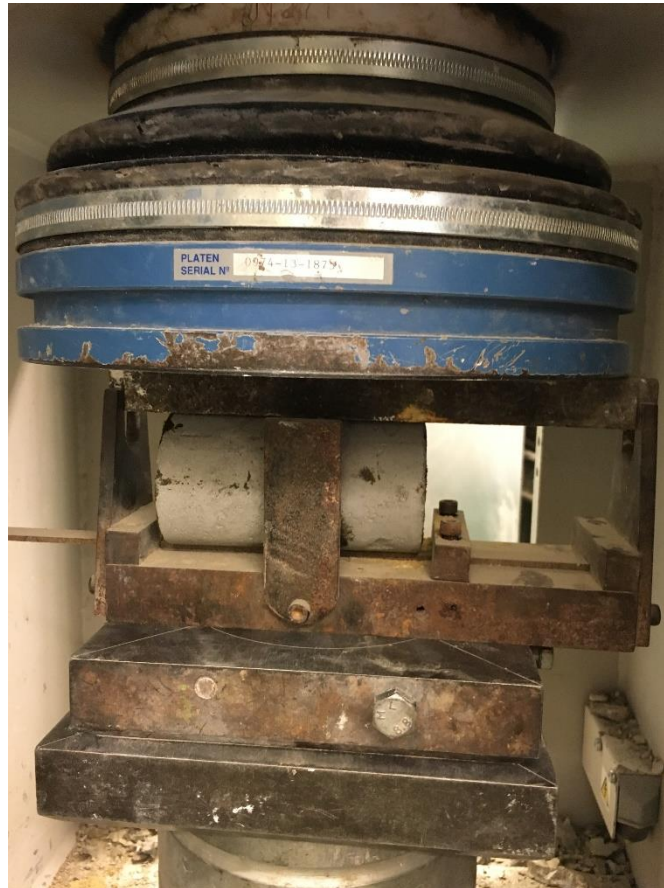
Figure 3-26: Indirect Tension Test
